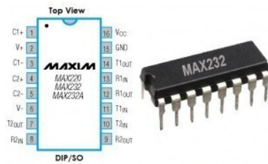
MAX232: Construction, Operation, Types and Application
